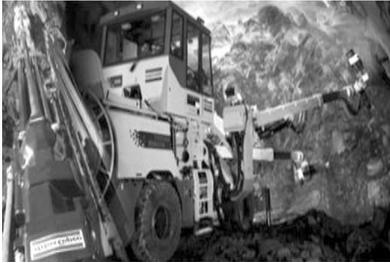
Photograph 1. The Jumbo Drill Rig
